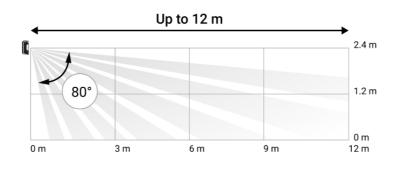
Vertical viewing angle of the detector
