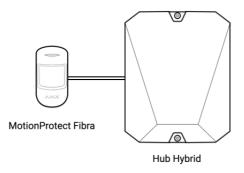
MotionProtect Fibra is a wired motion detector. Using an IR sensor, the detector can identify intrusions by detecting moving objects with temperatures close to that of the human body.
