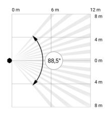
Horizontal viewing angle of the detector
