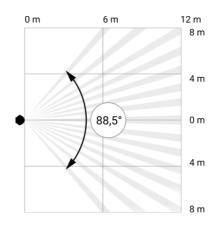
Horizontal viewing angle of the detector
