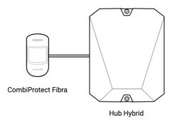
CombiProtect Fibra is a wired combined motion and glass break detector. In the armed mode, the detector instantly transmits an alarm signal to the hub when it detects motion or glass break. The hub, in turn, activates the sirens connected to the system, runs **scenarios**, and notifies users and the security company.
