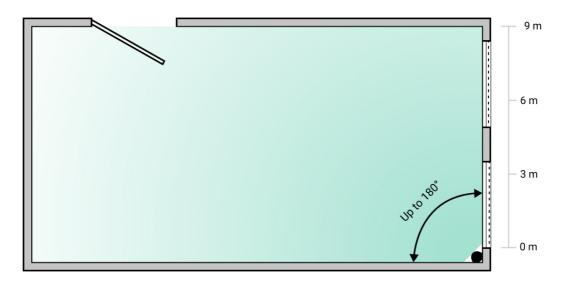
Detection angle of the glass break detector
