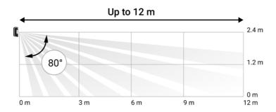
Vertical viewing angle of the detector
