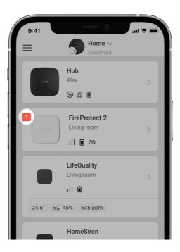
If FireProtect 2 malfunction is detected (for example, there is no connection with the hub), the malfunction counter is displayed in the device field in the Ajax
