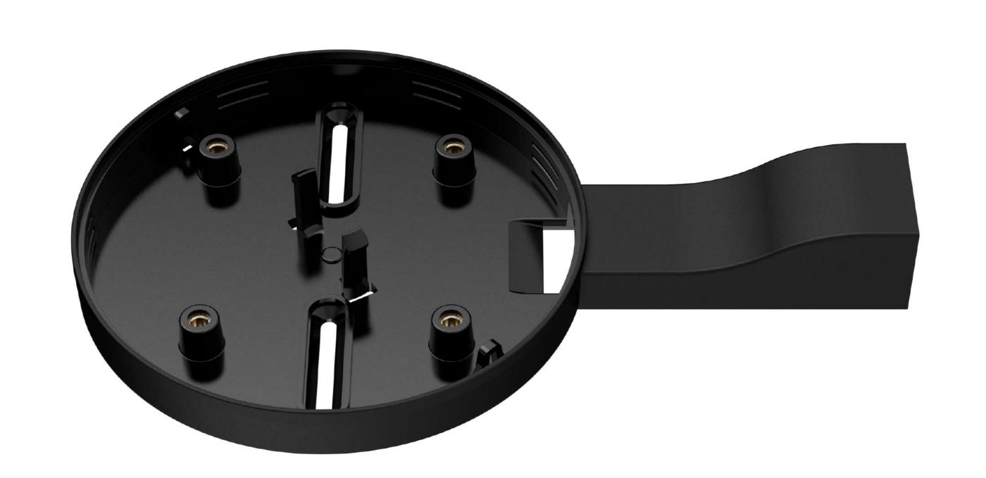
CableTrunk is an accessory designed for mains-powered FireProtect 2 AC detectors. It's a plastic connector for neat-looking wiring output that blends the detector into a standard cable tray. Using CableTrunk is ideal when it is impossible to run wiring inside the walls, as the connector provides an additional way to connect cables from two possible sides of the fire detector.
