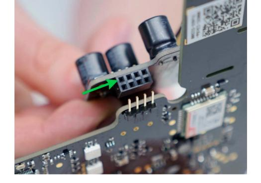
9. Reassemble the boards and the device body than tighten the screws.
