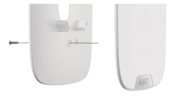
**11.** Fit the protective plastic panel in place (the Ajax logo on the connection side of the LED strip to the board) with little effort. The properly mounted plastic panel will protrude above the LED frame no more than 1.0 to 1.5 mm.
