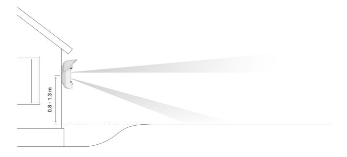
The detector should be installed on a flat, stable surface — for example, on the wall of a house or a solid fence. If the detector is installed on a shaky (unstable)
