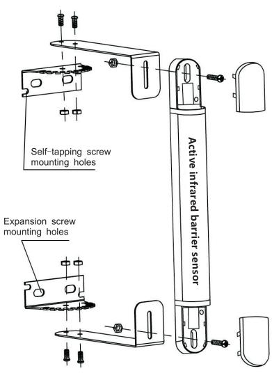
4.Note: one pair barrier sensor need two pairs brackets
